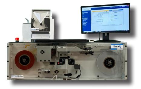
The intelliCount® Universal Automated Tablet/Capsule Feeder, patented by Pearson Medical, is specifically designed for the iPack® Rx Unit Dose Packager. This advanced technology offers a proven "touchless" solution for automated Unit Dose Packaging, ideal for longer packaging runs. Utilizing vacuum technology, it eliminates the need for customized, drug-specific calibrated canisters, making it a fully automated packaging solution for any pharmacy.
